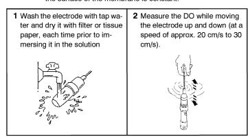
Note>>> The electrode membrane is thin and easily torn. Place it into solution slowly.
