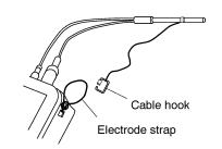
Note▶▶▶ Be sure to attach the cable hook to the electrode strap. If not, the cable may break
