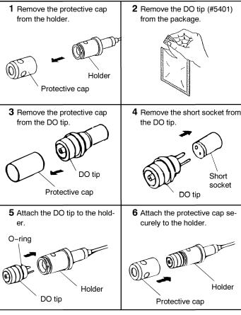
Note▶▶► Do not dispose of the short socket that was removed. It is necessary when storing the electrode.
