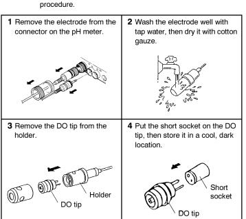
Note▶▶▶ Avoid storing the electrode in hot place or places with high humidity. Store the electrode indoors, out of direct sunlight.
